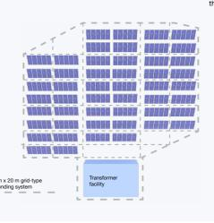
Grounding system 3: Ground grid: If a grid-type grounding system is installed, the IEC 62305-4 standard recommends 20x20 m as the correct size.
